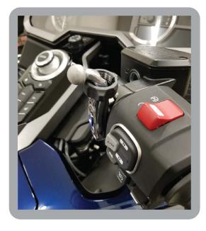
2. Snap your drink holder onto the ball and thread the large plastic nut back onto the drink holder. Adjust the angle, tighten it down, and you are ready to go.
